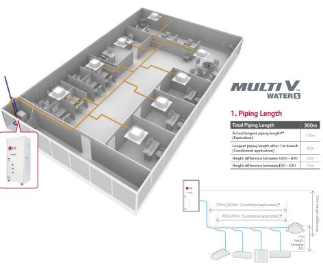
\* Assume equivalent piping length of Y branch to be 0.5m, that of header to be 1m, calculation purpose.
